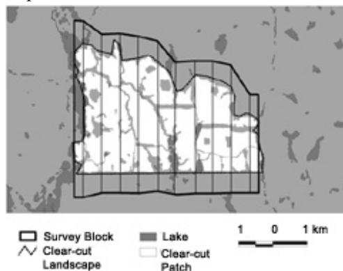
Fig. 3. Aerial survey plan for a clear-cut landscape. North-south transects are spaced 0.5 km of longitude (600 m) apart.
